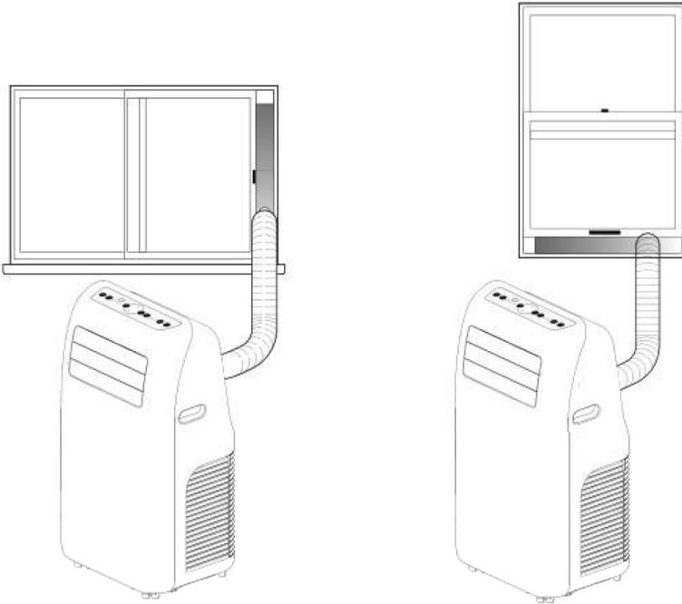
**NOTE:** The length of the exhaust duct is variable between 480 mm and 1500 mm (adaptors included). Using a shorter length of ducting uses less energy.
