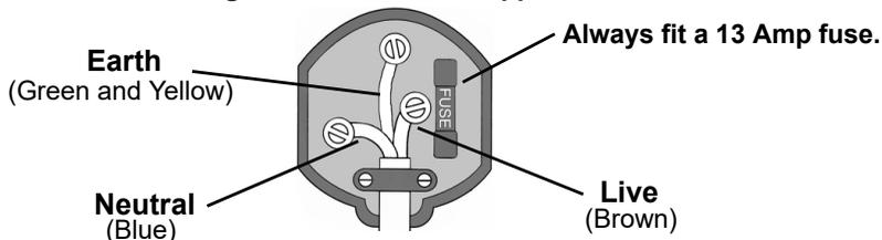
**Ensure that the outer sheath of the cable is firmly held by the clamp**
