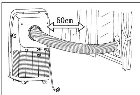
3. Screw the air exhaust duct on to the air outlet located on the rear of the air conditioner.
